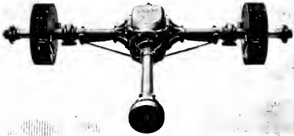
American Rear Axle—Two Sets of Expanding Brakes.
